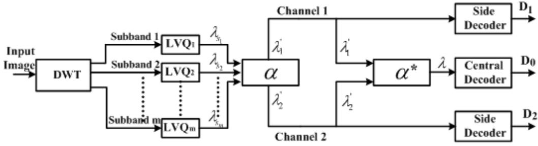
Figure 1. Block diagram of our scheme
