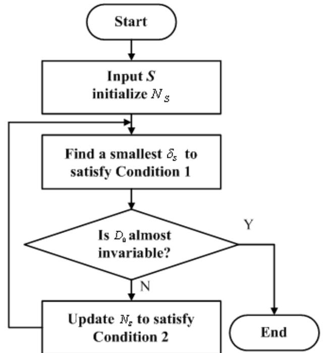
Figure 3. The flow chart of optimization algorithm
